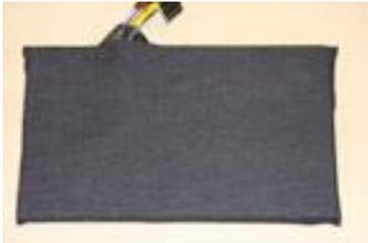
**Figure 1.** The TWEND device, which can be held by both hands on each side for the physical deformations.
